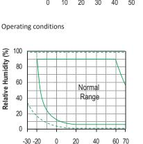
Long term exposure to humidity levels outside of the 'normal' range may temporarily offset RH measurements (±3%RH after 60 hours). Once returned to less extreme conditions the device will slowly return towards calibration state.
